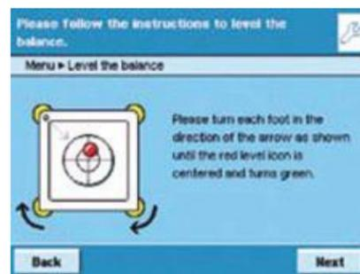
Figure 1 - Diagram showing the new-generation Sartorius Cubis balance with assisted leveling on the display.
